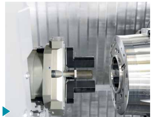
3-axis workpiece handling for flange parts
