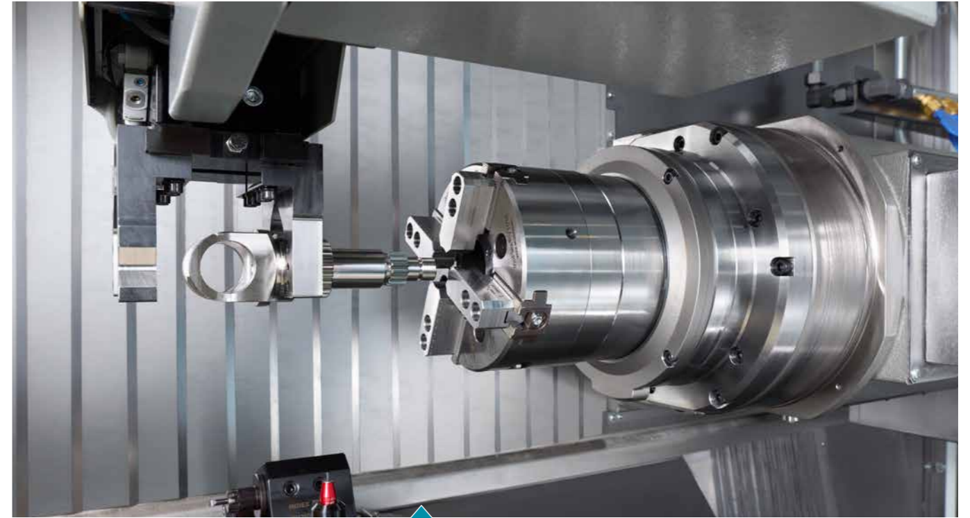
Removal of finished parts (or feeding) using a workpiece-specific gripper for shaft or flange parts
